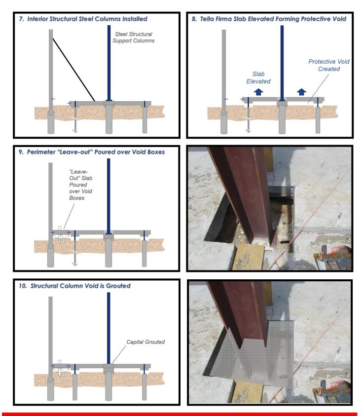
SlabTek System in Tilt-up Wall
