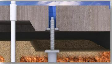
3. The slab is raised to the proper height by turning the bolt. The protective void allows for soil expansion
