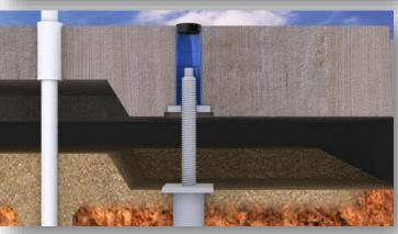
4. The plastic finishing cap is installed and mortar is placed on top of the cap to match to the slab floor finish
