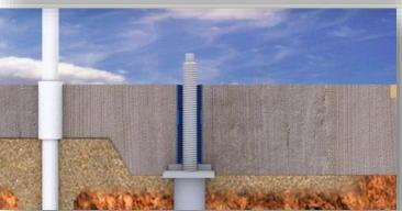
2. The concrete is poured. The plastic sleeve keep concrete out of the mechanism thread area
