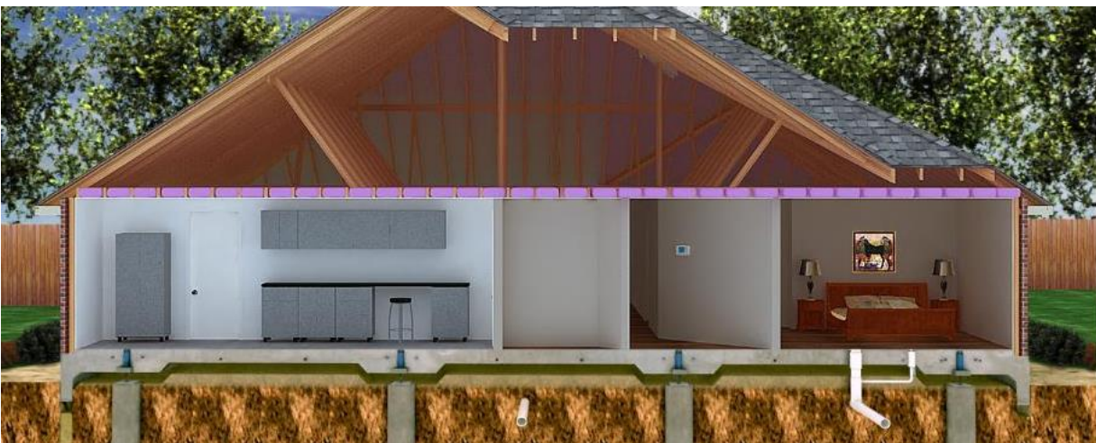
The lateral load capacity of a SlabTek foundation is determined by the lifting mechanism array
