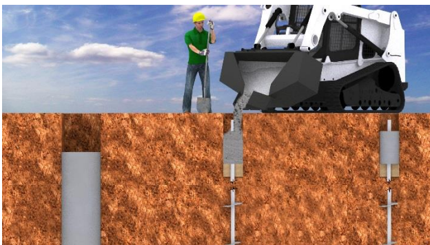
3. Helical Pier Caps Poured
