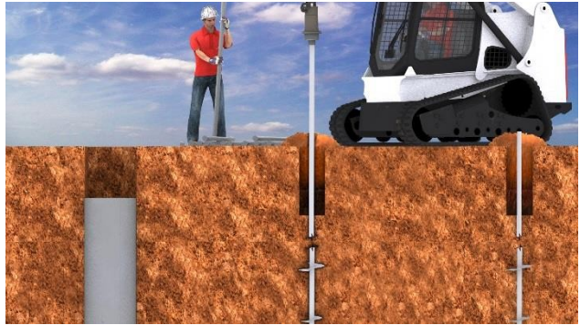
24" Dia. Concrete Piers and 2" Dia. Steel Helical
