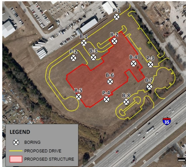
Diagram showing location of geotechnical borings
