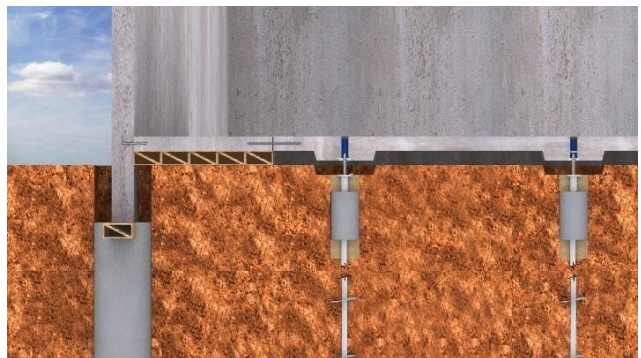
Pour strip is poured and tied into the slab and panels.
